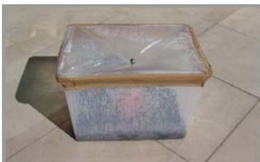
5. Place the solar still in a still and sunny location (it may pay to check with groundsmen to find the best position – wind can cause the cling wrap to flap about so that the droplets miss the cup).
