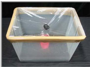
4. Seal the tub with cling wrap and tape. Add a pebble or large marble directly above the cup forming a depression for the water droplets to roll down.
