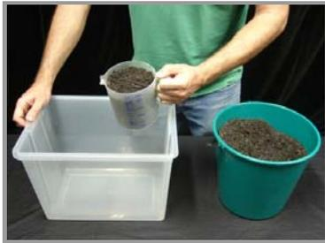
1. Add one or two litres of soil or sand to the plastic tub – if making more than one still, add the same amount of soil or sand is used in each. You should also ensure the soil has a consistent and uniform moisture content.
