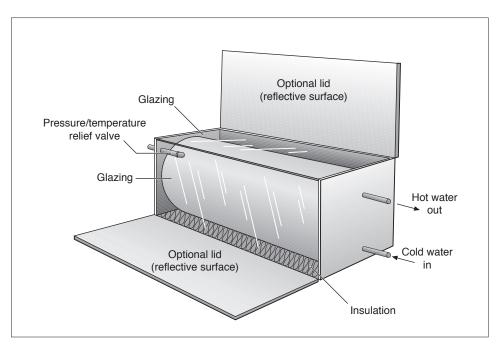
**BREAD BOX OR BATCH HEATER** The basic, passive water heater allows cold water to flow in from the bottom and hot water to flow out of the top.
