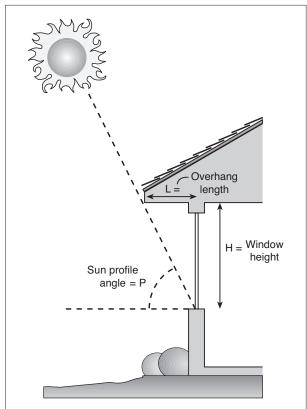
FIG. 2. Sizing overhang
