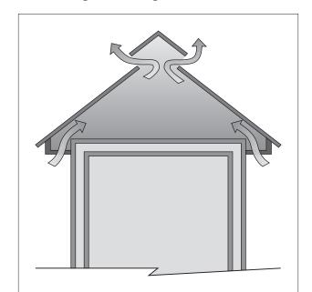
FIG. 3. Ridge and soffit vents
