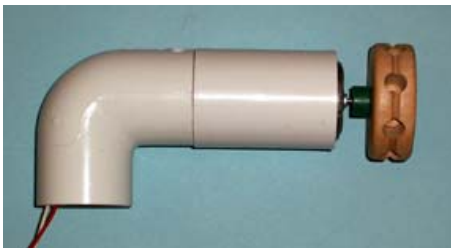
Nacelle complete with Tinkertoy Hub!
