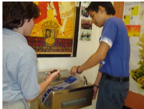
To calculate the flow rate (gallons per minute or GPM) of a faucet, water fountain, or shower, use a flow meter bag. Detailed instructions are provided on the bag.
