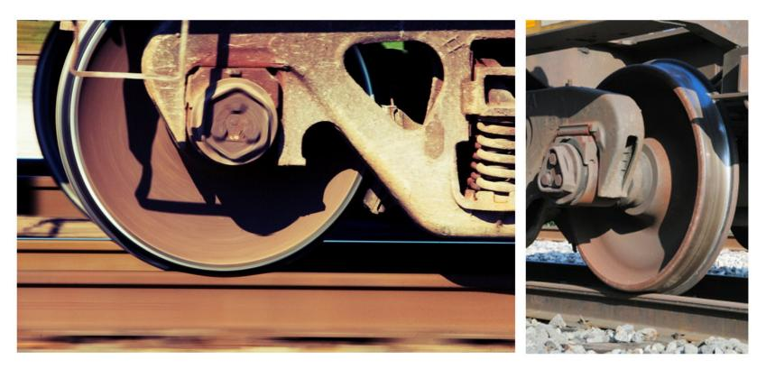
Trains also have some eco-friendly designs. For example, they have steel wheels that move on steel rails. This design reduces the amount of rolling friction, as compared to rubber car tires on paved roads. And so, these trains require less fuel to run.
